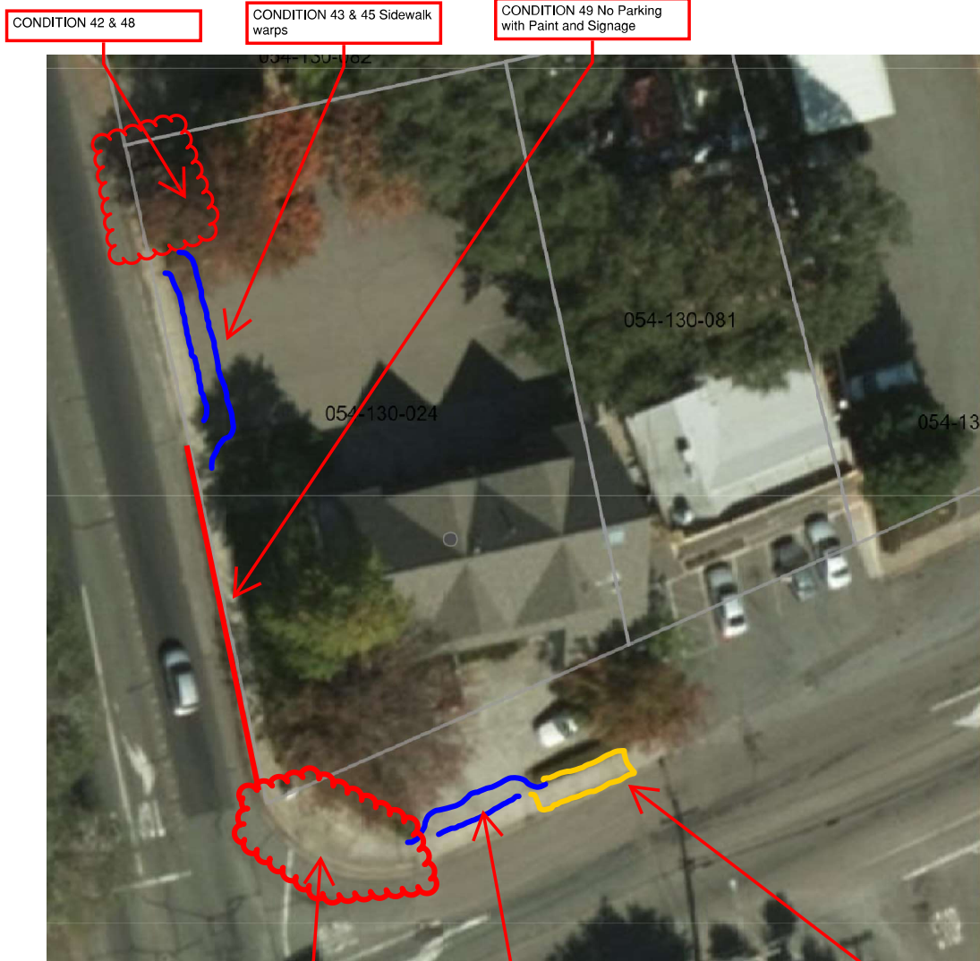
CONDITION 42 & 48 Bus Stop and barricade. Check (e) tree for conflict 6-foot wide pad behind sidewalk.
