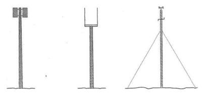
The silhouette is a calculation of the physical surfaces of the combined tower and antenna(s) included in a telecommunication facility. Only the physical surfaces, and not the air spaces in between, are counted in the calculation. The silhouette calculation is measured from the viewing angle which presents the largest exposure from an elevation perspective.
