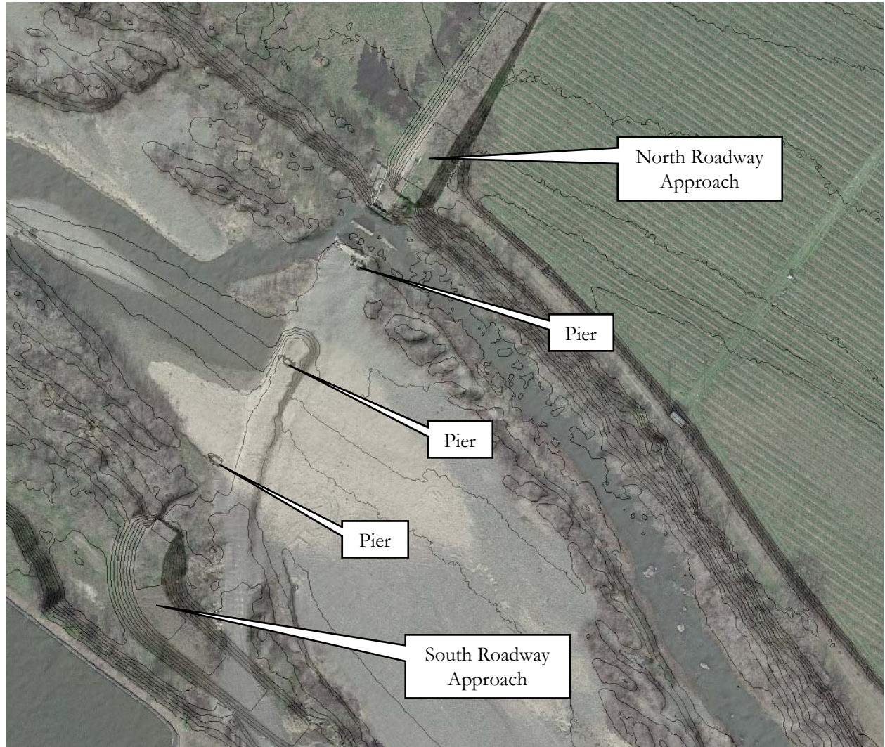
Figure 10. DEM used for proposed 500 ft long bridge.
