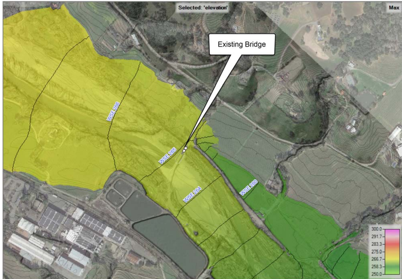
Figure 13. Water surface elevation results for existing conditions
