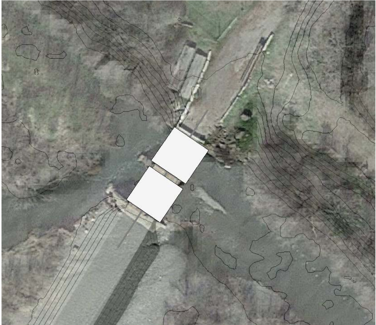
Figure 8. Existing bridge modeled as double box culvert (plan view).
