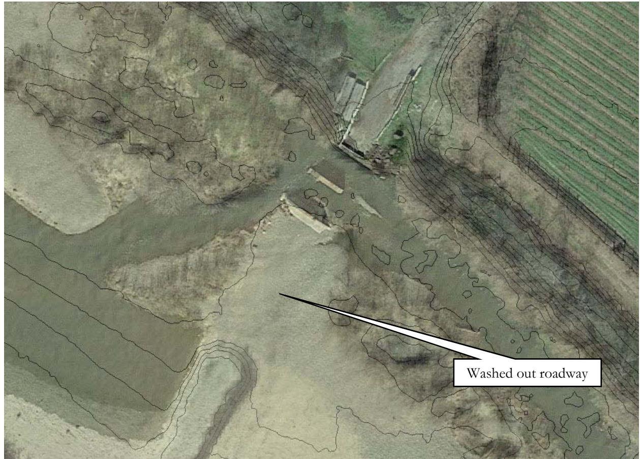
Figure 6. Close up of DEM at the existing crossing (2 ft contours shown).
