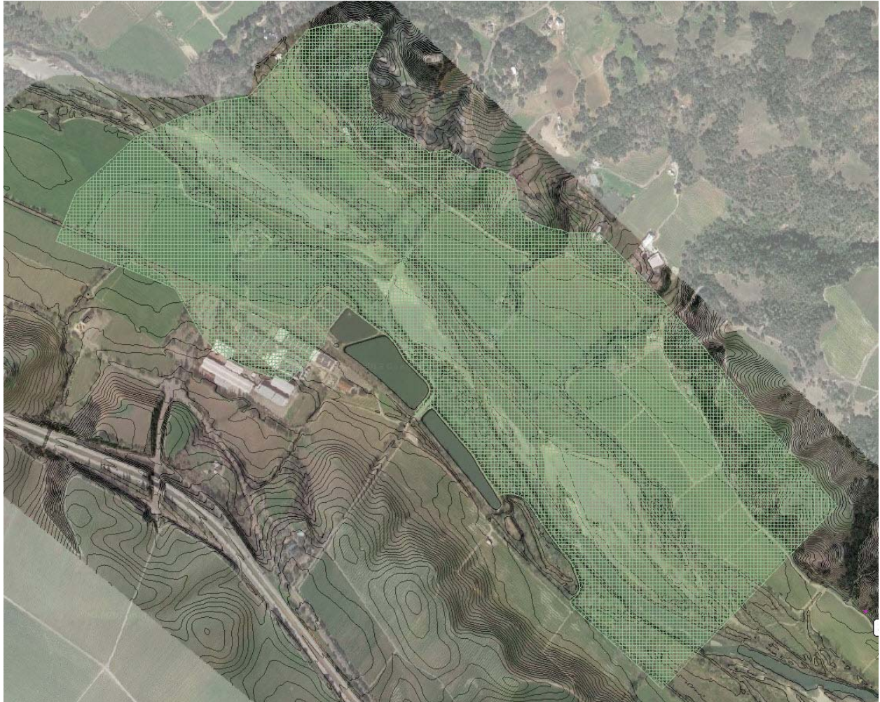
Figure 5. 2D Flow Area used for analysis.
