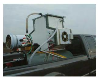
Fig. 2. The mobile odour generator mounted in the box of a pick up truck.
