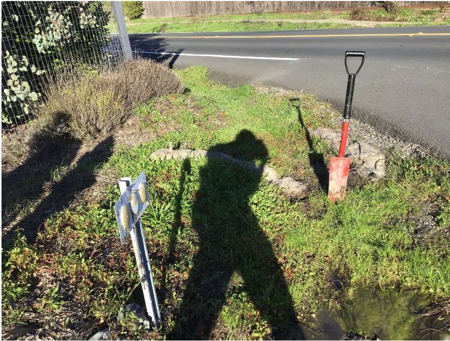
Photo 16. Sample Point 5 (SP05). Sample point is located in a ponded area within the lowest point within a roadside ditch near a culvert and immediately adjacent to straw wattle.
