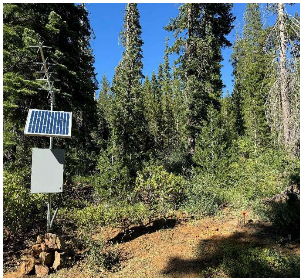
Figure 3: Example of a fully installed USGS soil moisture station in the Feather River Basin in Plumas National Forest (left); example of a soil pit with a tape measure and 5 installed soil moisture sensors (right).
