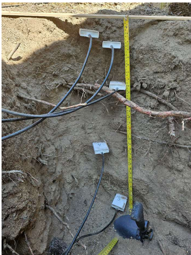
Figure 3: Example of a fully installed USGS soil moisture station in the Feather River Basin in Plumas National Forest (left); example of a soil pit with a tape measure and 5 installed soil moisture sensors (right).
