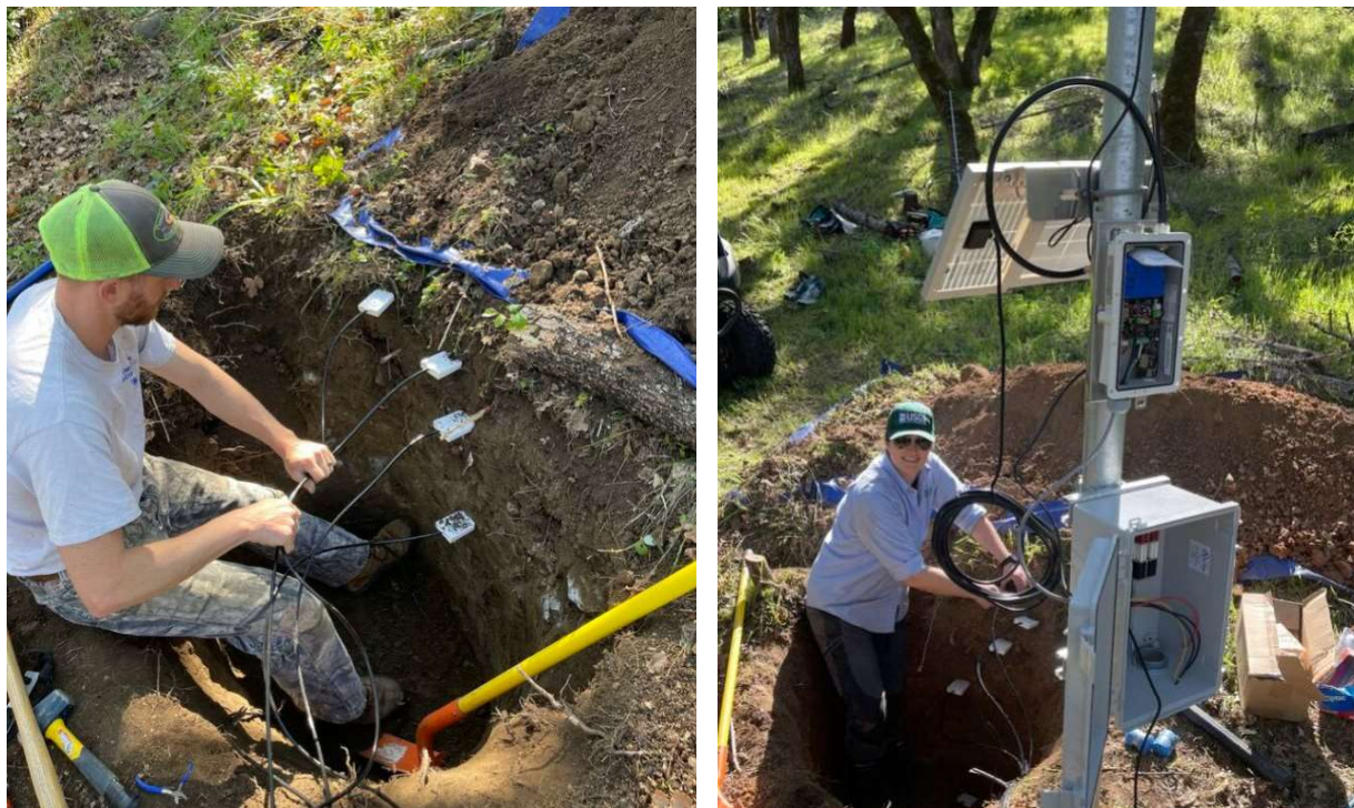
Figure 2. Example of a USGS soil moisture monitoring station under construction at the Pepperwood Preserve; Ryan Ferrell, Pepperwood Foundation Hydrologist (left), Michelle Stern, USGS Hydrologist (right).
