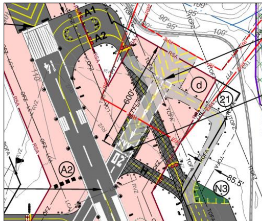
Figure 3 – Proposed Runway 20 End Relocation and Extension
