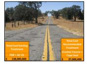
with cape seal on rural local roads could potentially save up to \$100 million when compared with current treatments i.e. full depth reclamation and overlay (see graphic).
