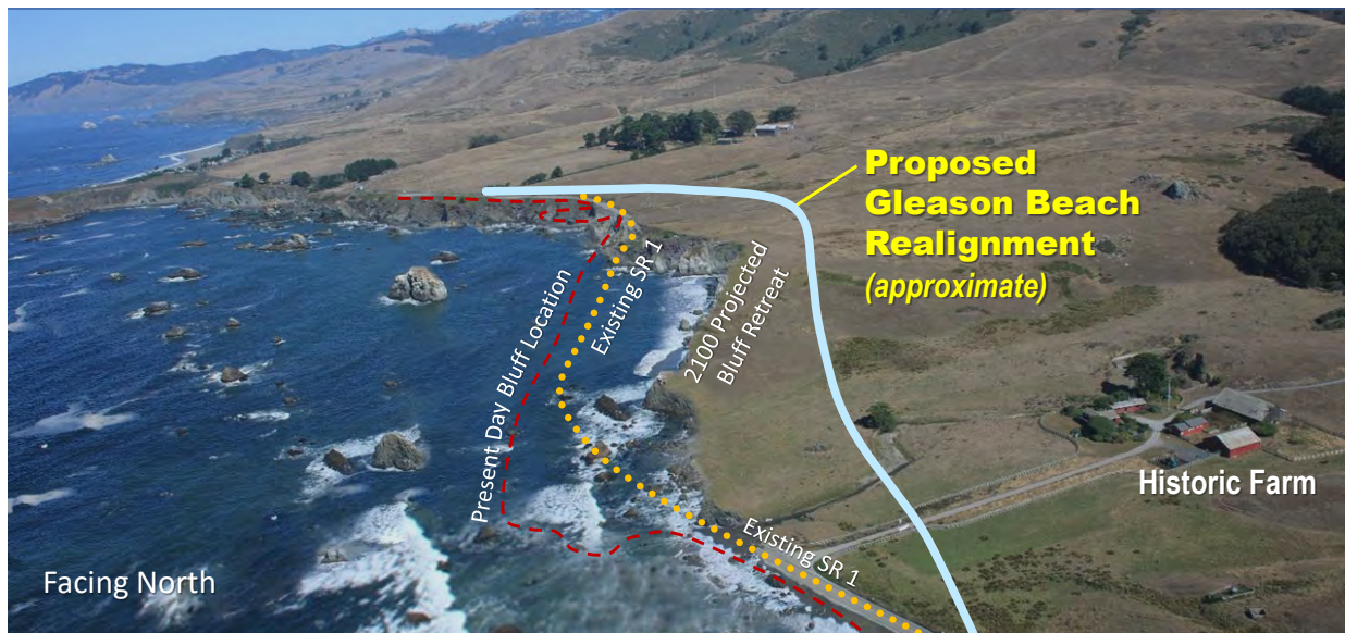
Visualization of possible bluff retreat scenarios in relation to approximate highway alignments. 2
