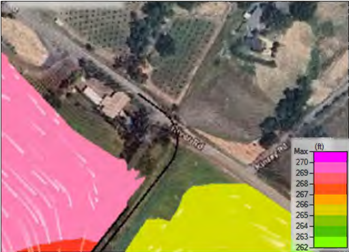
Figure 8 – Flood Extents Parcel 117-080-012 – Proposed Conditions
